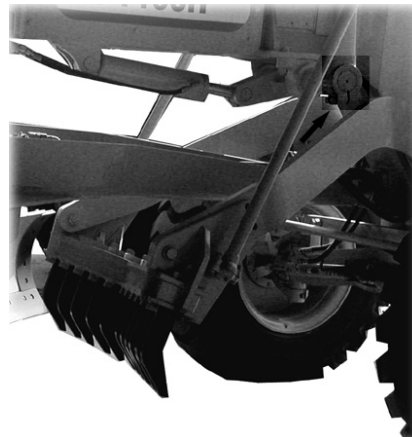
12. Blade lift cylinder ball joint (2 points)
