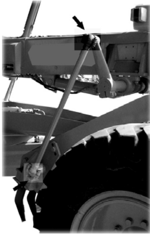
9. Scarifier cylinder pin (2 points)
