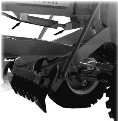
11. Blade lift cylinder yoke (6 points)
